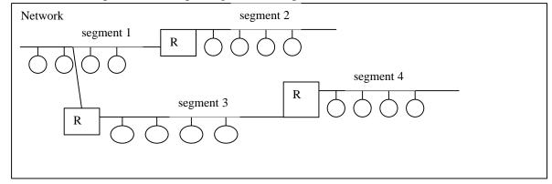
PROFIBUS allows up to 32 nodes per segment and up to 126 nodes for one network.
